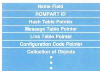
Fig. 2. Structure of a ROMPART.
