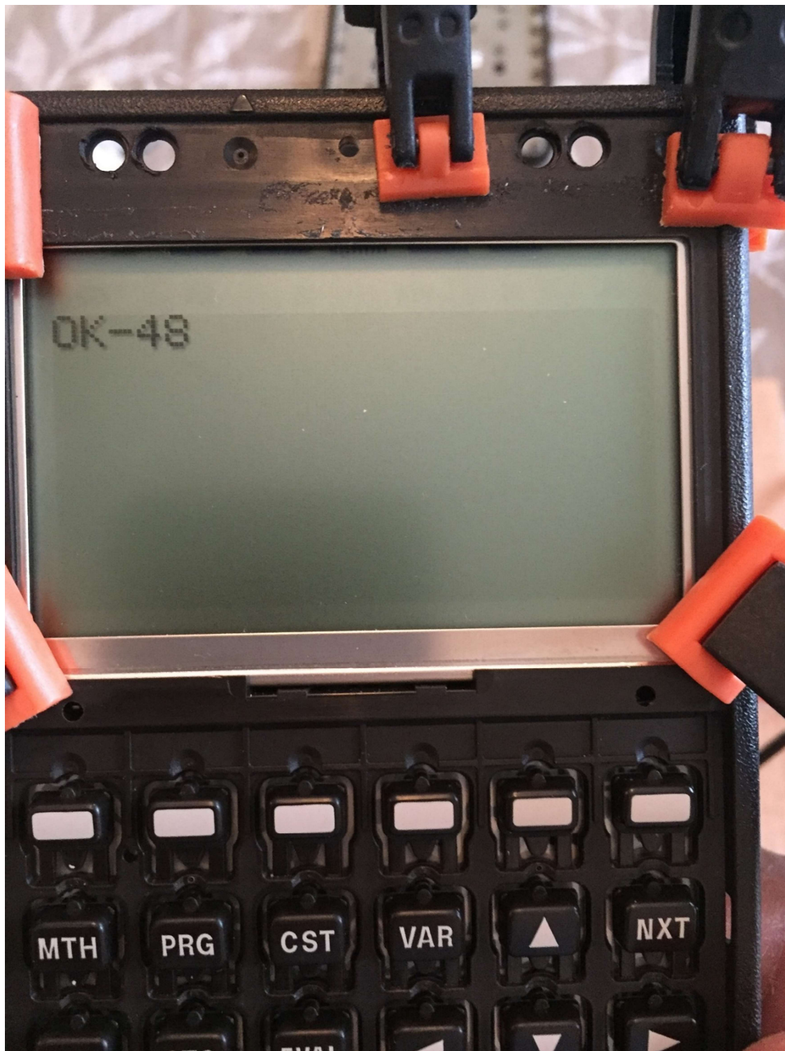
HP 48sx self test passes! I actually verified the IR send/receive, printing, and card slots while the PCB was still attached using the plastic clamps.
