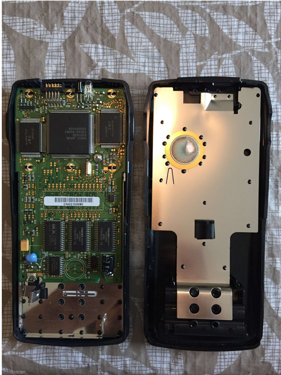
The 39G is very similar to the 48sx under the hood
