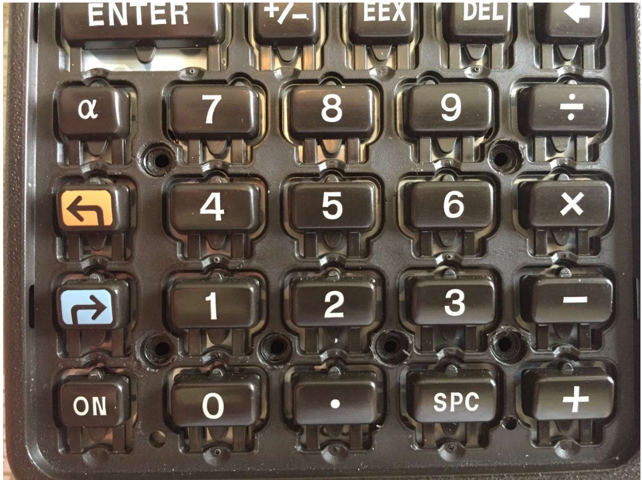
Putting the halves back together. Note that the rivets are not popped in place yet.
