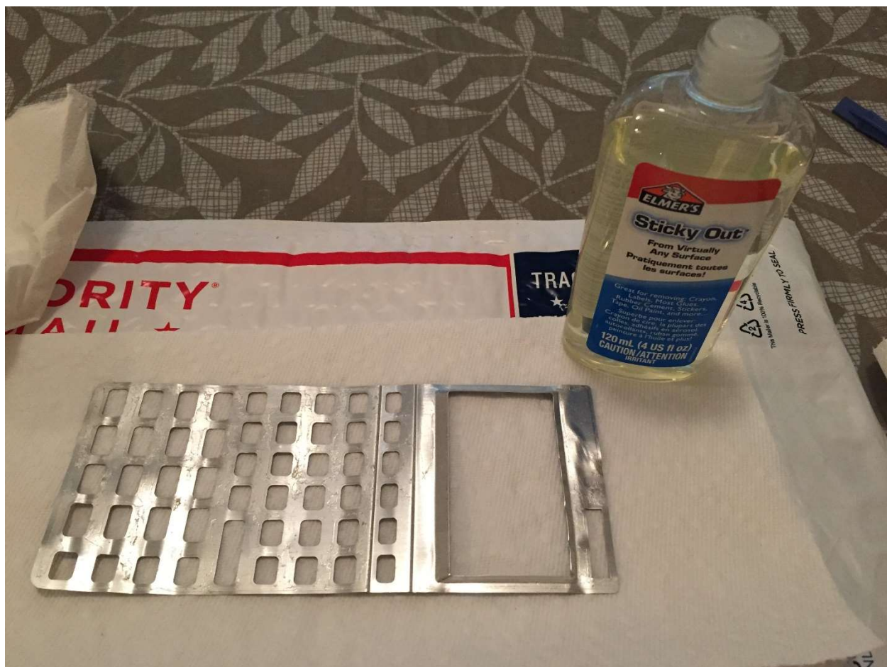
Adhesive remover to get the glue off the overlay
